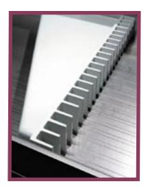
Spring-loaded Backgage Fingers Every backgage finger is spring-loaded to prevent
