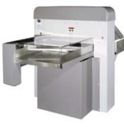
**Rear Safety Cover** The see-through rear safety cover prevents reaching into the cutting area from behind while providing a clear view of the backgage. It also keeps the cutter table free of debris.
